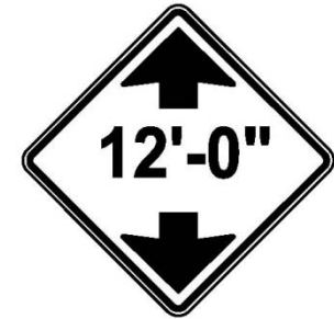
CLEARANCE SIGN DETAIL W12-2
